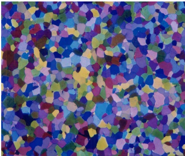
a) Motor Lamination Steel (original 100X)
